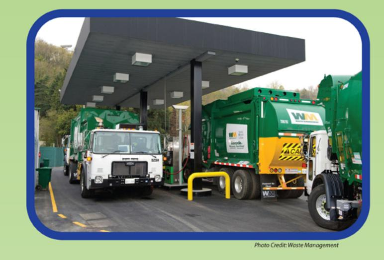
As garbage decays, it releases methane. Trash companies capture that gas, chill it until it liquefies, and use **liquid methane** to power their trucks.
